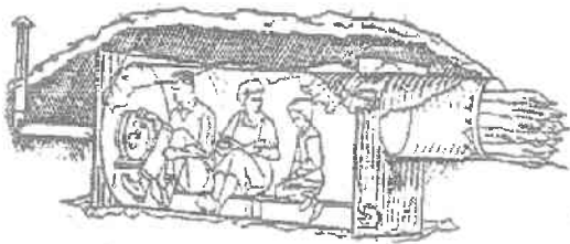
Belowground Corrugated Steel Culvert Shelter
